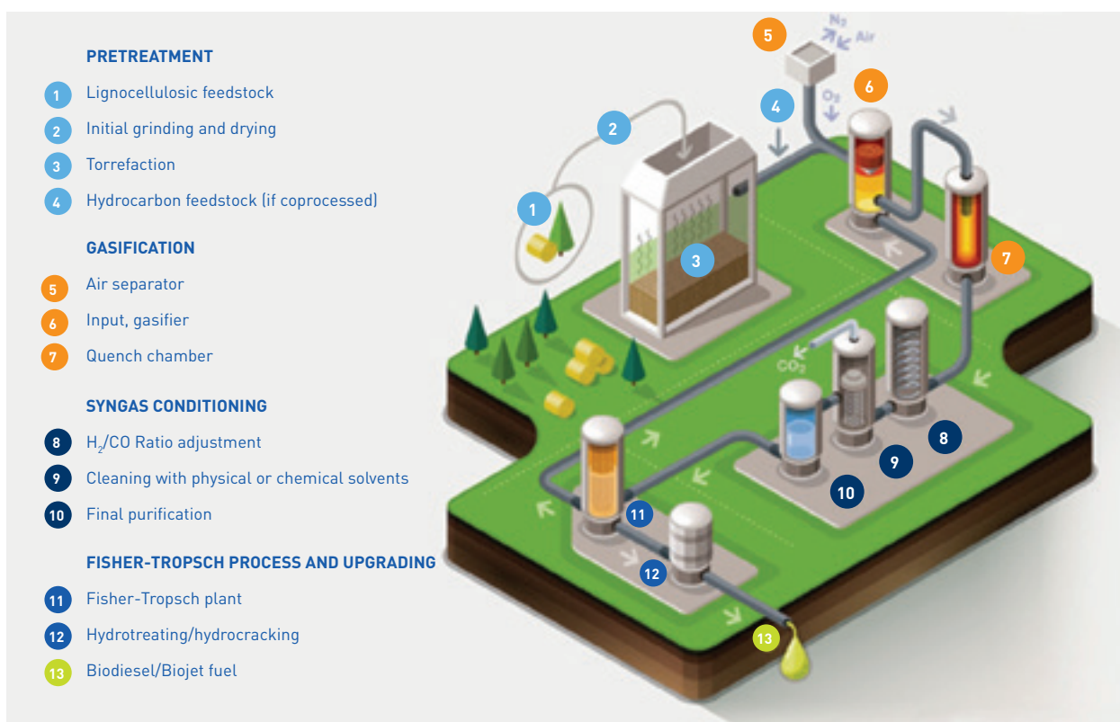
FIGURE 10: BioTfuel, A PROJECT TO PRODUCE BIOFUELS VIA THERMOCHEMICAL CONVERSION
