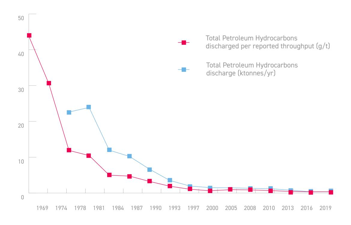
The EU refineries have significantly improved the quality of refinery water effluent in the last decades. The amount of Total Petroleum Hyrdrocarbons (TPH) discharged in effluents from reporting installations continued to decrease to extremelly low levels relative to pre-1990; both in terms of the absolute amount of TPH discharged and the amount expressed relative to the volume of feedstock processed (throughput) and the refining capacity of the installations.
