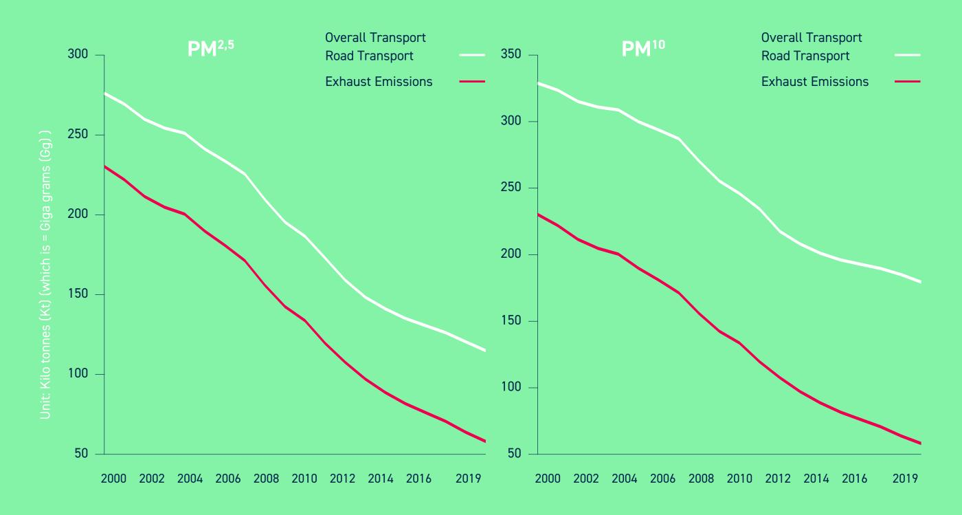
Particulate Matter (PM) emissions are continuously decreasing as the result of cleaner diesel fuel, advanced engines and effective emissions control technology. Since the introduction of the Euro 6 standard, modern road vehicles with diesel engines are using highly efficient filters that remove 99.9% of PM.
