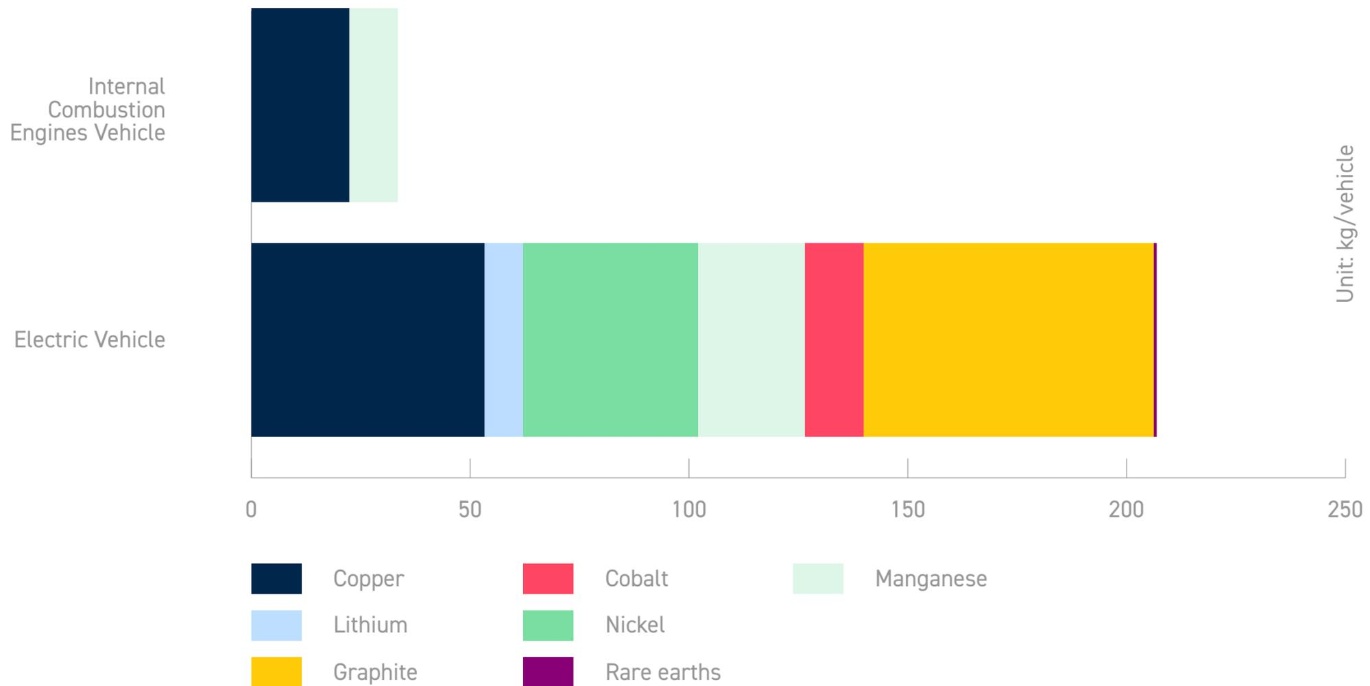
A typical electric vehicle (EV) requires six times the mineral inputs of a conventional car. Lithium, nickel, cobalt, manganese and graphite are crucial to battery performance, longevity and energy density, whereas rare earth elements are essential for permanent magnets that are vital for EV motors. The shift to EVs is set to drive a huge increase in the requirements for these minerals, meaning that the energy sector is emerging as a major force in mineral markets.
