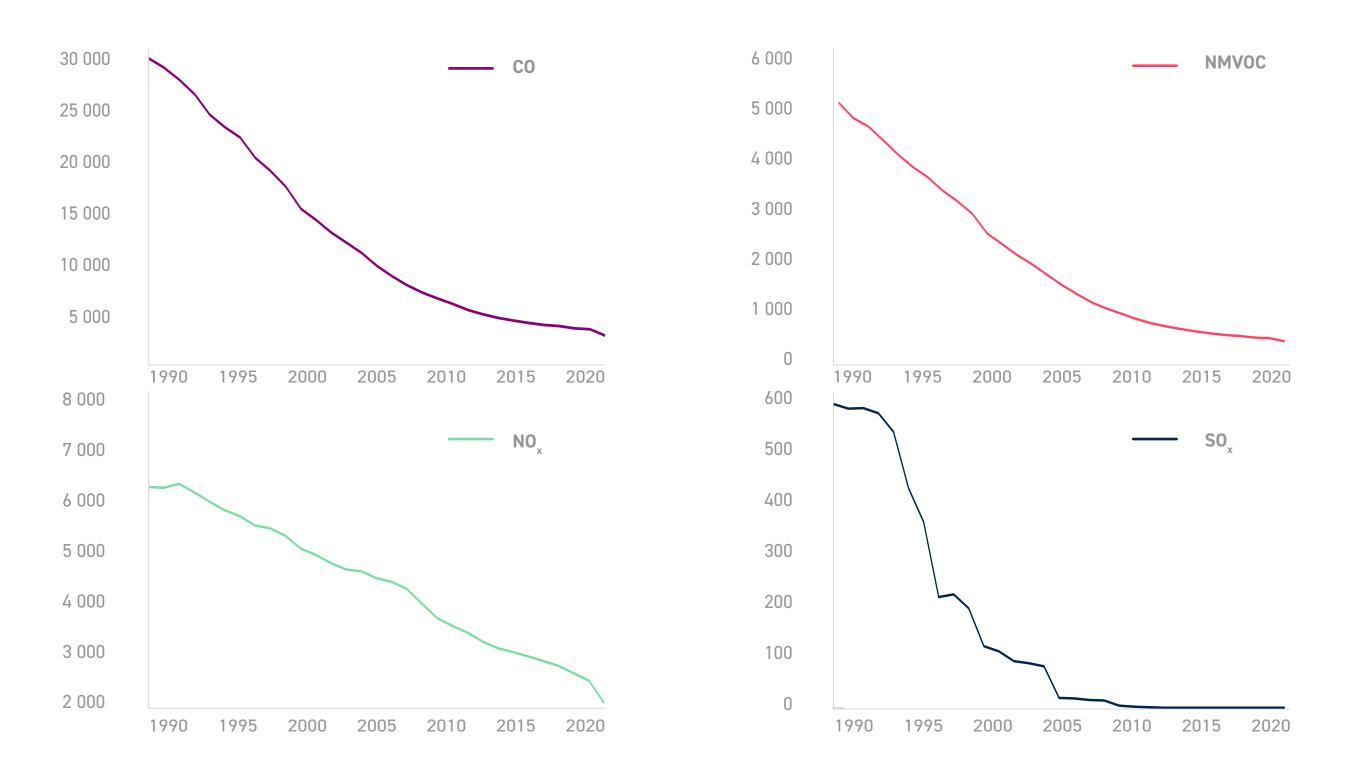
Since 1990, the refining industry has contributed to cleaner exhausts by today containing over 80% lower  $SO_x$ , NMVOC & CO, while  $NO_x$  emissions decreased by over 60%. These significant improvements are the result of the partnerships with the automotive industry aiming at improving the fuel-engine efficiency and leading to multiple environmental benefits.
