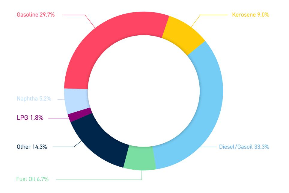
A wide range of products, from transportation and industrial fuels to chemical feedstock, are produced from crude oil. EU refineries also produce many specialty products, such as bitumen for road construction and roofing, lubricants for transport and industry, petroleum coke for the metal industry as well as waxes, solvents and other specialised products. Fuels for transport represent the biggest share of the production. **Note:** Please note that due to rounding, figures may not add up.
