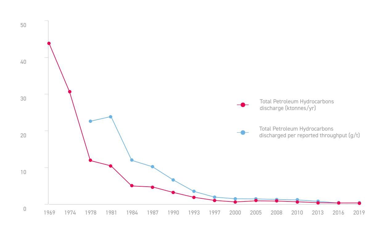
The EU refineries have significantly improved the quality of refinery water effluent in the last decades. The amount of Total Petroleum Hyrdrocarbons (TPH) discharged in effluents from reporting installations continued to decrease to extremelly low levels relative to pre-1990; both in terms of the absolute amount of TPH discharged and the amount expressed relative to the volume of feedstock processed (throughput) and the refining capacity of the installations.
