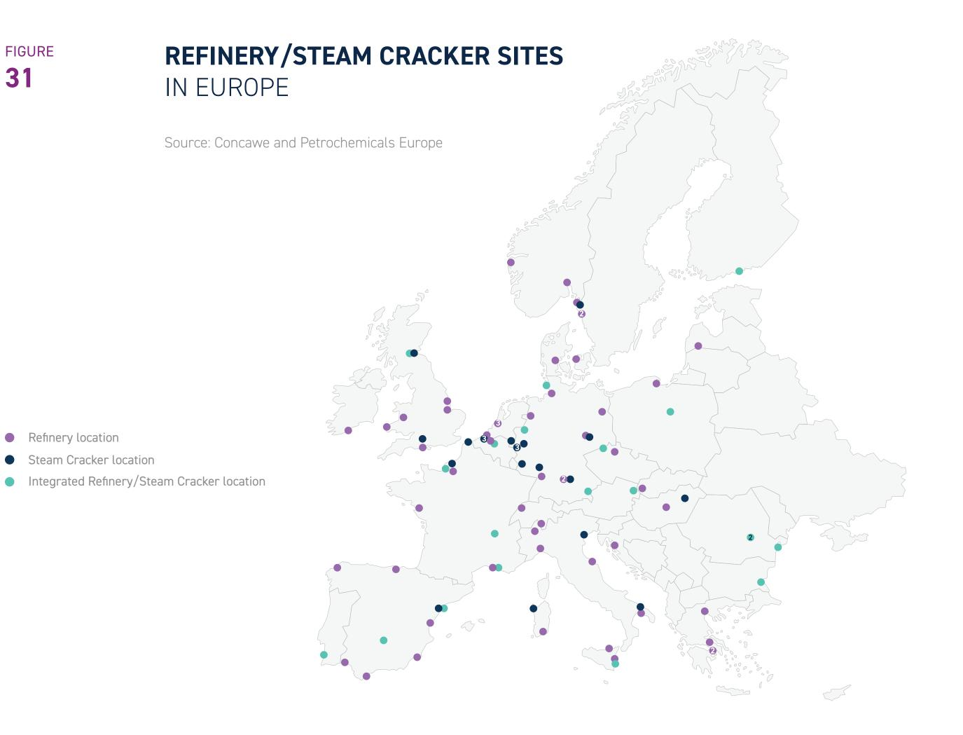
A large number of refineries are integrated with, or very close to steam crackers which produce the feedstock for the petrochemical industry. Such interconnections show how refining is an intrinsic part of the industrial value chain and provides the basis for advanced high value products.
