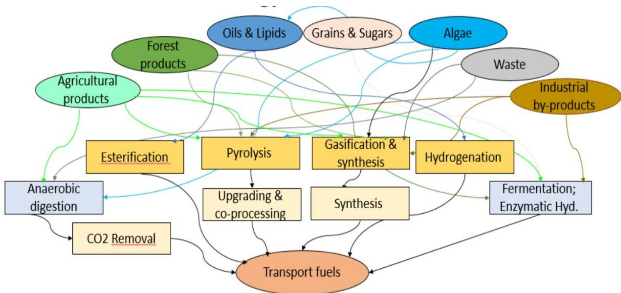
Figure 28: The complexity and flexibility of biomass value chains via conversion technologies and intermediate steps
