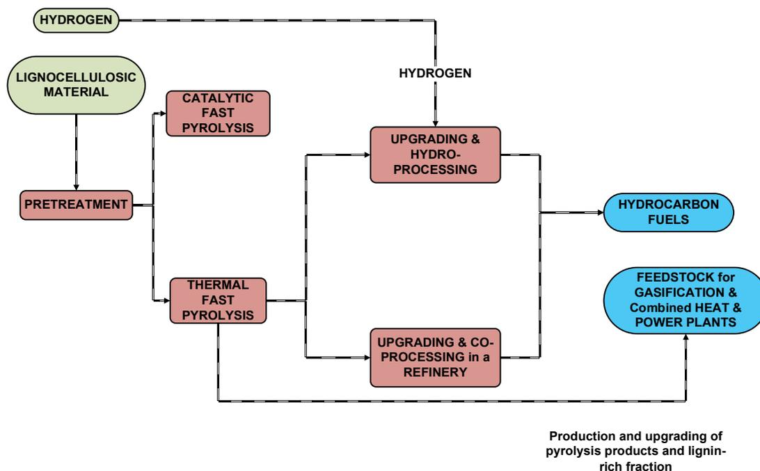
Figure 44 Simplified process flow diagram for pyrolysis. Process flowsheet also shows upgrading to hydrocarbon fuels or co-processing in a refinery.
