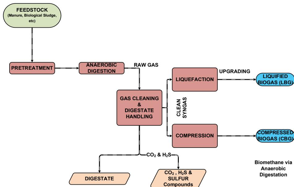
Figure 39 Simplified process flow diagram for biomethane from anaerobic digestion<sup>104</sup>
