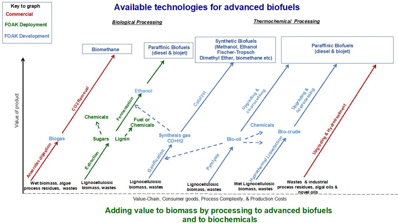
Figure 26: Simplified schematic for technologies and value chains for advanced biofuels<sup>3</sup>
