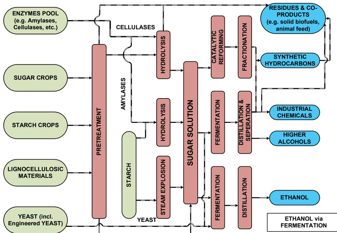
Figure 40 Ethanol, higher alcohols, industrial chemicals & hydrocarbons via sugar extraction from biomass and fermentation<sup>12</sup>
