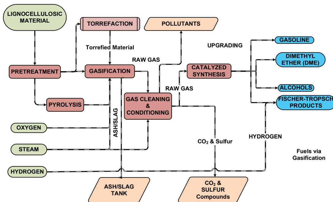
Figure 41 Fuels, industrial chemicals & hydrocarbons via biomass gasification and synthesis<sup>12</sup>
