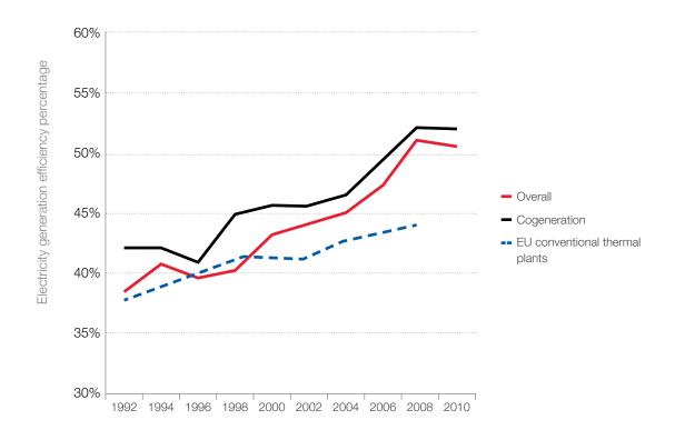
Refineries have long recognised the considerable efficiency gains offered by cogeneration, which now accounts for more than 90% of the electricity produced in EU refineries.
