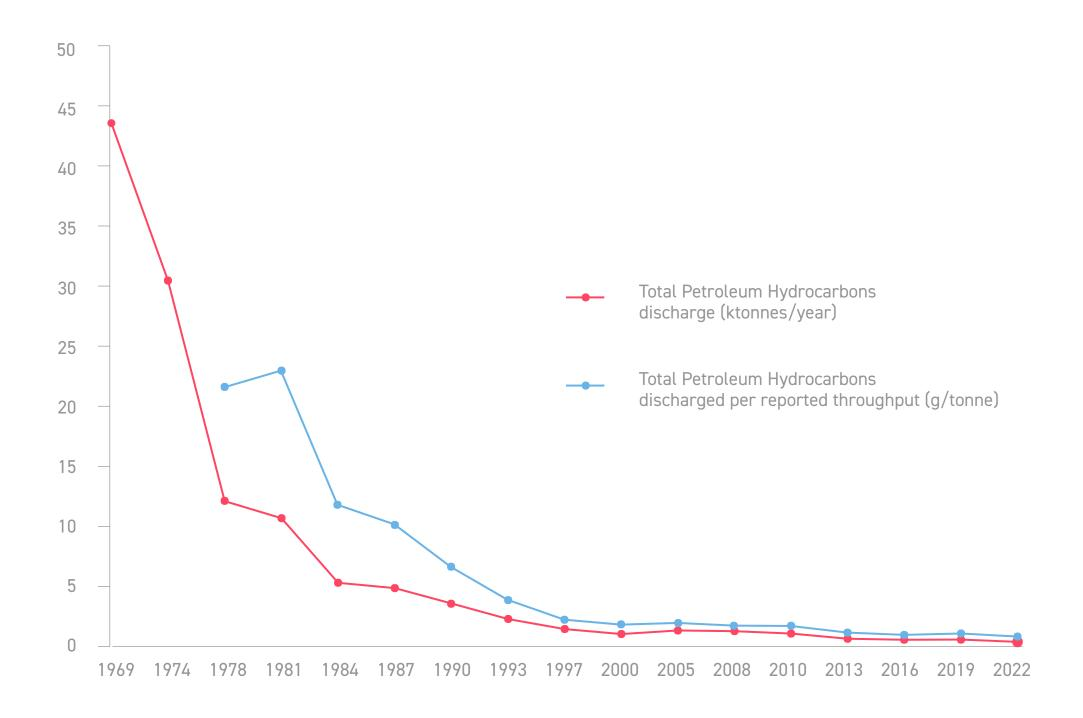
EU refineries have significantly improved the quality of refinery water effluent in the last decades. The amount of Total Petroleum Hyrdrocarbons (TPH) discharged in effluents from reporting installations continued to decrease to extremelly low levels relative to pre-1990; both in terms of the absolute amount of TPH discharged and the amount expressed relative to the volume of feedstock processed (throughput) and the refining capacity of the installations.
