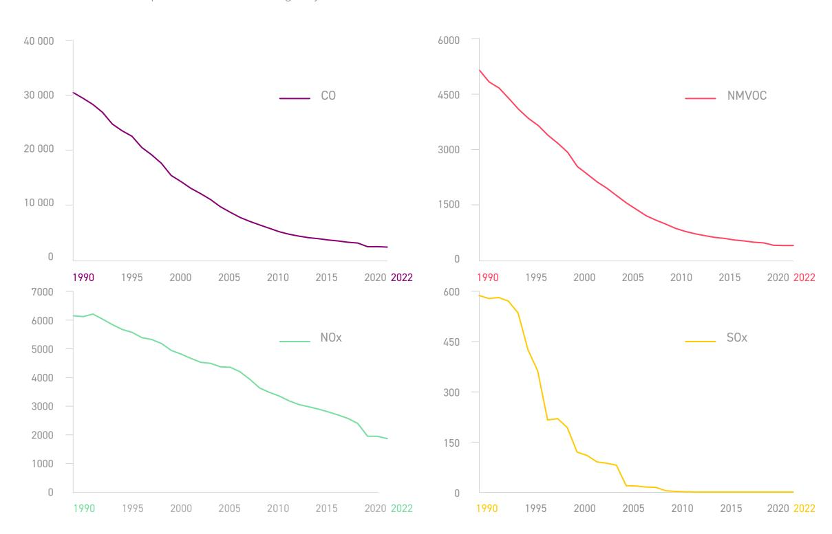
Since 1990 the refining industry has contributed to cleaner exhausts by today containing 99% lower SOx, over 90% lower NMVOC & CO, and 62% lower NOx emissions.
