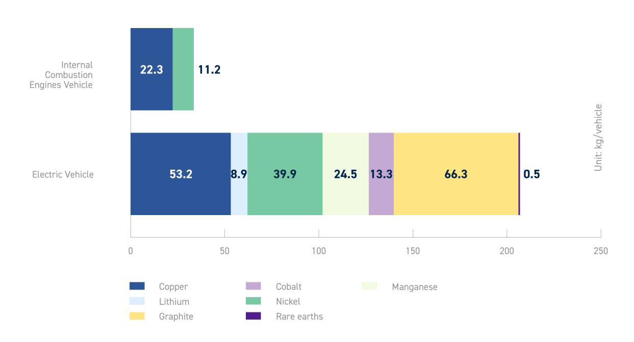
A typical electric vehicle (EV) requires six times the mineral inputs of a conventional car. Lithium, nickel, cobalt, manganese and graphite are crucial to battery performance, longevity and energy density, whereas rare earth elements are essential for permanent magnets that are vital for EV motors. The shift to EVs is set to drive a huge increase in the requirements for these minerals, meaning that the energy sector is emerging as a major force in mineral markets.
